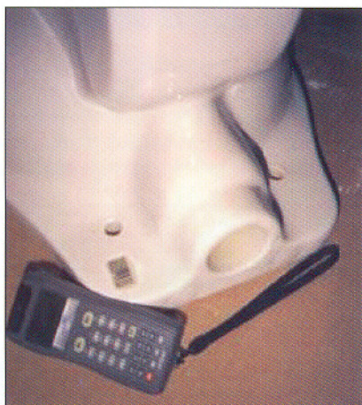
Fig. 2 - Bar code system for production management.
