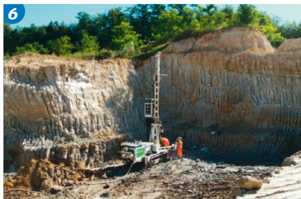
Figs. 6-7 • Geological prospecting with rotary core drilling equipment
