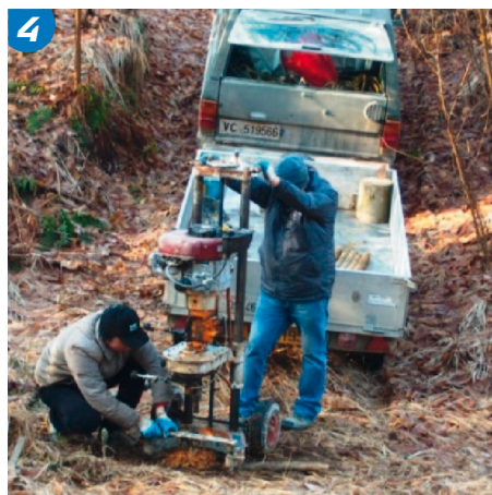
Figs. 4-5 • Geological prospecting with mechanical auger drilling equipment
