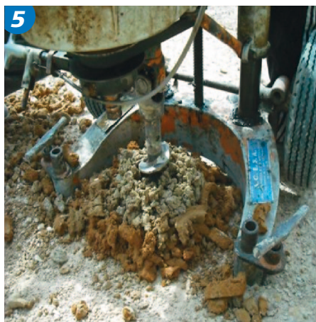
Figs. 4-5 • Geological prospecting with mechanical auger drilling equipment
