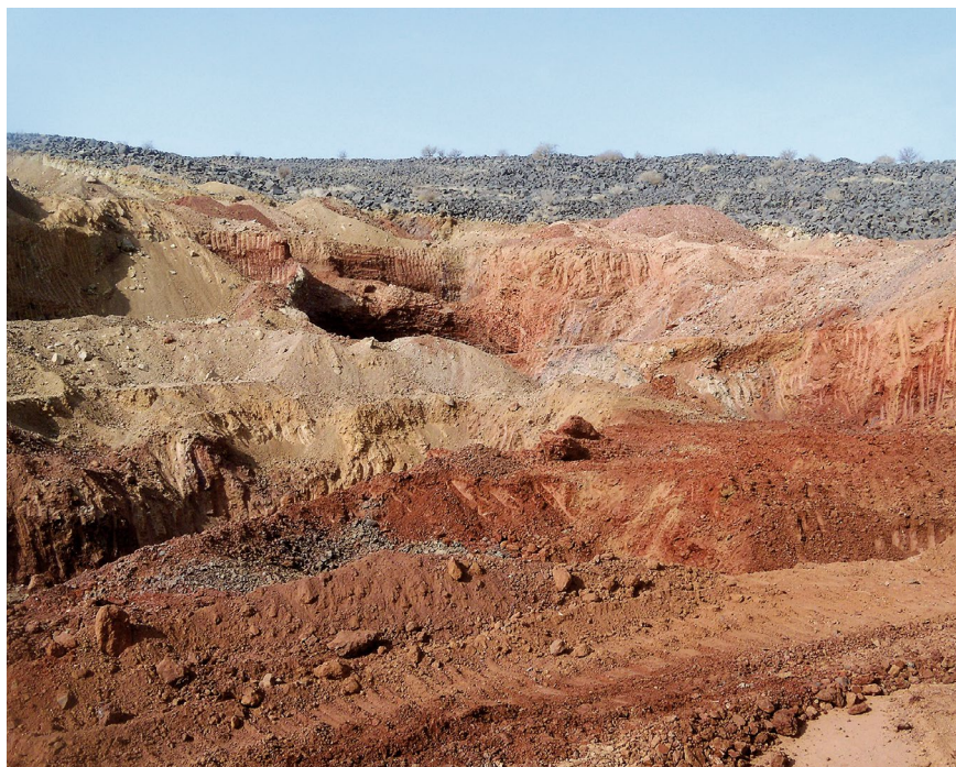
Figure 7 Example of red-firing plastic clays mining (Jeddah, Saudi Arabia). (© Bertolotti)
