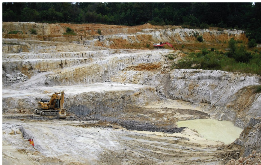
Figure 6 Example of: medium-low plasticity white-firing clay mining (Italy). (© Bertolotti)
