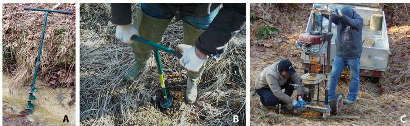
Figure 5 Preliminary clay sampling: manual auger (A, B) and sampling with a motorized auger (C). (© Bertolotti)
